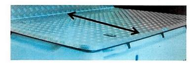
Removable rear lid on remainder of load bin manufacture from aluminium tread plate with a suitable tubular frame and two T-handles.
